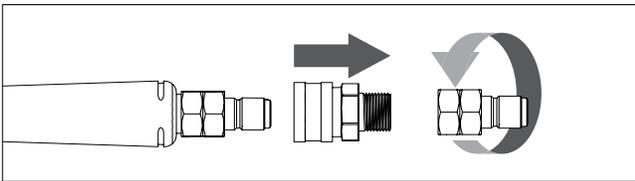
3. Securely tighten remaining male quick-connect fitting onto attachment handle.
