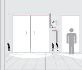
Foam pattern: Up to 9x5 ft. Foam pattern: Up to 8x4 ft. Foam pattern: Up to 6x3 ft. at each nozzle Spray tip: ST8060-12SS
